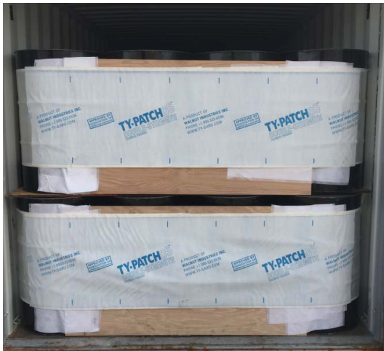
Photo 2: Doorway area showing the rear section of the load secured with Ty-Gard DS, and \frac{3}{4} inch plywood.
