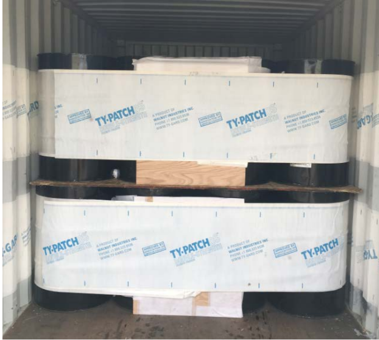
Photo 1: First 50 drums secured with 24 inch Ty-Gard DS, and \frac{3}{4} inch plywood.
